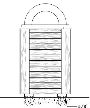
5/8" (16 mm) DIA. HOLES PROVIDED FOR ANCHORS BY OTHERS. (TYPICAL-4)
